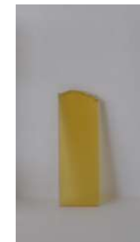
MPA cured epoxy
