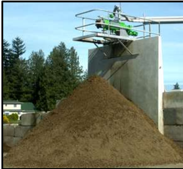
Dairy Manure AD: Fiber, P-rich fine solids, ammonia sulfate solution
