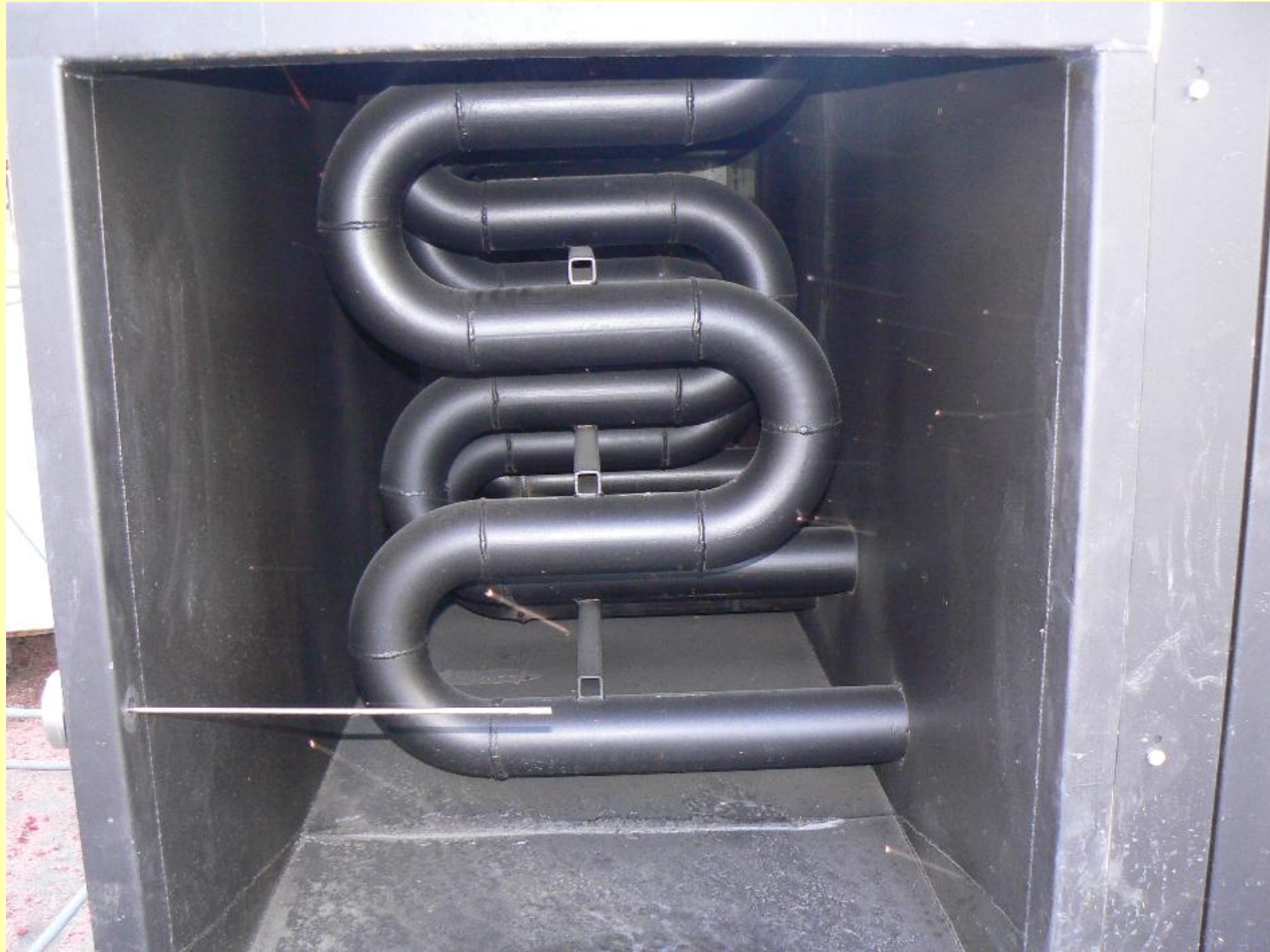
inside air-to-air heat exchanger
