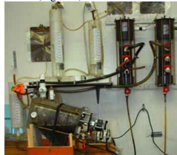
Figure 3: Experimental High Solids Anaerobic Digestion System
