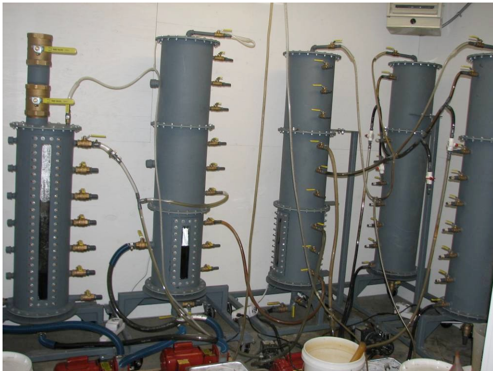
Figure 42. The floor scale moderate solids anaerobic digestion system.
