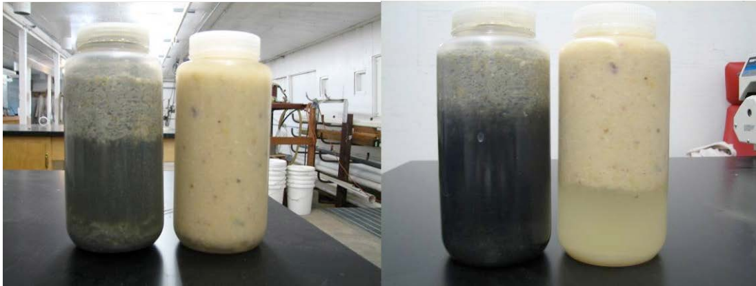
Figure 47. Natural separation of liquid and solid in a mixture of food waste and inocula from the effluent of UASB seed reactors (left bottle), and food waste and water (right bottle). (Left picture: after one day, Right picture: after two days).
