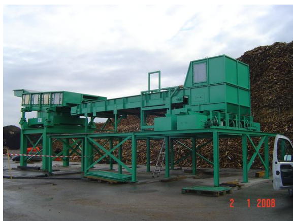
Figure 42. Oscillating screen used to separate different sized biomass ( http://www.sf-gmbh.de/screening-plants/oscillation-screening-machines/?album=5&gallery=62 &nggpage=2 ).
