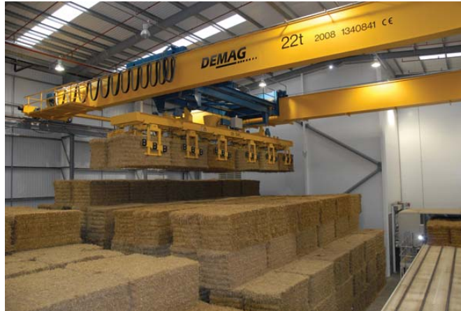
Figure B1. Cranes used for handling bales in power stations ( http://warehousenews.co.uk/?p=6326 ).
