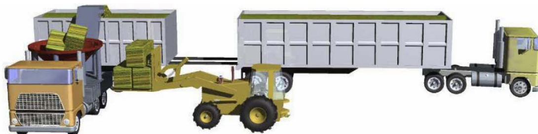
Figure 25. Grinding bales into chips for transport (Tagore and Hess 2005).
