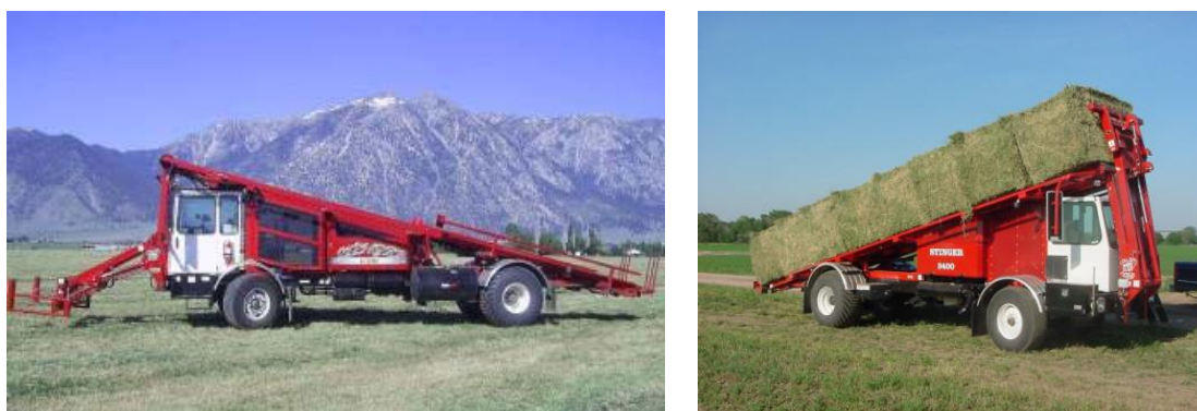
Figure 28. Stringer stackers for bales recollection. (source: http://www.stingerltd.com/index-1.html , http://www.usagnet.com/manufacturers/85/3400.jpg ).
