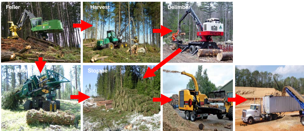
Figure 18. Supply chain for forest thinning (Sources: http://www.deere.com/en_US/cfd/forestry/deereforestry/media/images/landing/stories/909j-feller-buncher-2-lg.jpg ; http://www.johndeere.com/en_US/cfd/forestry/deere_forestry/info_center/feature_stories/pf_harvesting-energy.html ; http://www.unb.ca/standint/nbcc/machine/other/Peart_Jennith.htm ; http://en.wikipedia.org/wiki/File:Europe_Chippers_1.jpg )
