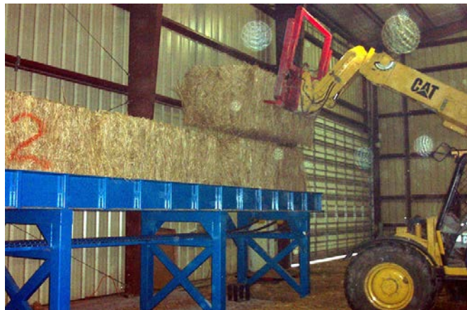
Figure B2. Bales loaded on a conveyor using a wheel loader ( http://iowaswitchgrass.com/cofiringcycle~processing.html ).
