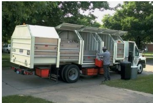
Figure 6. Compartmentalized recycling truck (Source: Treehugger web site: http://www.treehugger.com/files/2008/11/celebrate-zero-waste-day.php ).
