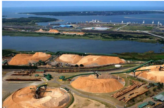
Figure A3. Radial stackers (Source: http://www.ports.co.za/news/article_2008_04_13_1946.html ).
