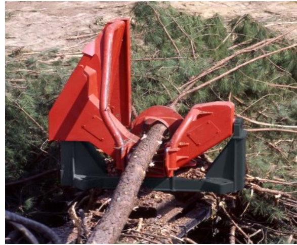
Figure 20. Delimiting and debarking using a flail (Source: http://www.ansonvillefire.com/site_flash/320cMed.jpg ).
