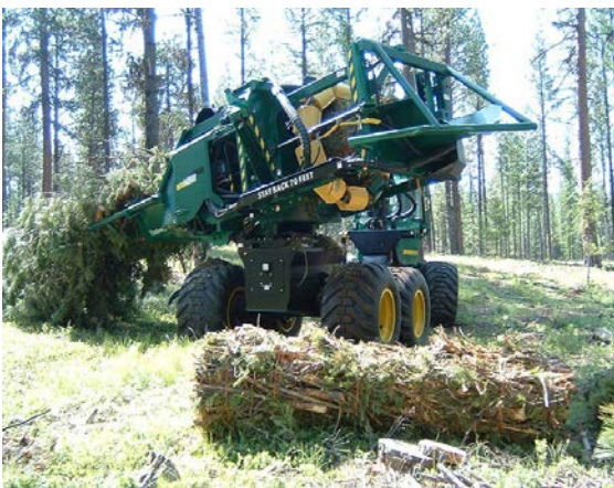
Figure 21. Wood bundler baling forest residues (Source: ); and slash bundles at roadside (Source: http://www.deere.com/en_US/cfd/forestry/deere_forestry/media/flash/photogallery/energy_wood_harvestor/1490d/index.html and http://www.unb.ca/standint/nbcc/machine/other/Peart_Jennith.htm ).
