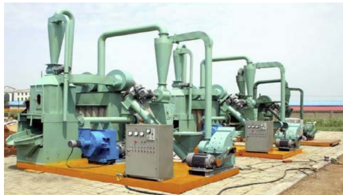
Figure 35. Transportable pelletizers (IMG Pellets Systems) (Mason et al., 2009).
