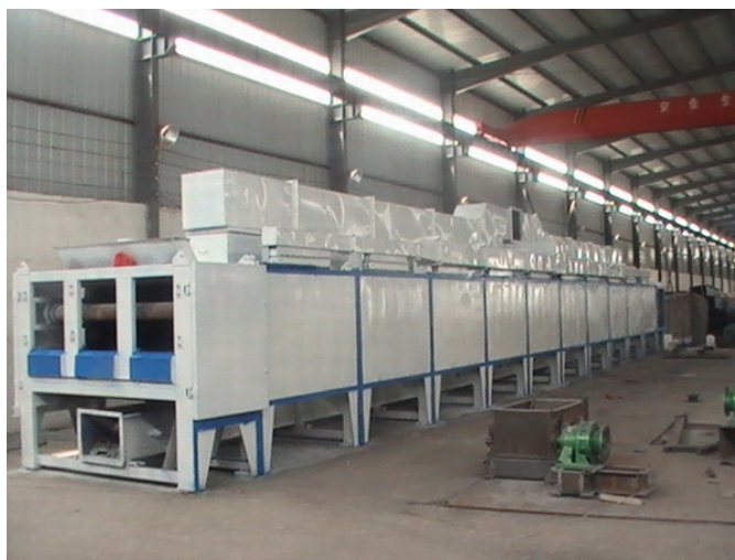
Figure C3. Perforated band conveyor drying system ( http://www.lp-machinery.com/en/ Products Details .aspx ).
