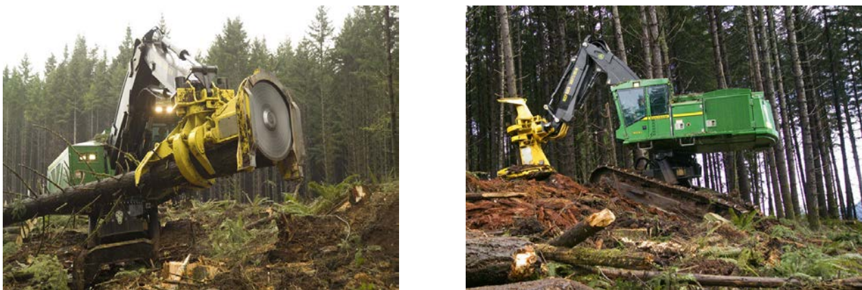
Figure 19. Feller buncher with grappling device and disk (source: http://www.deere.com/en_US/cfd/forestry/deere_forestry/track_fellerbunchers/deere_fellerbuncher_selection.html ).
