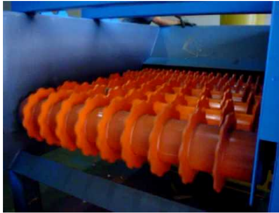
Figure 43. Disc screen used to separate different sized biomass ( http://greenbd.info/screen+wood+chips/ ).
